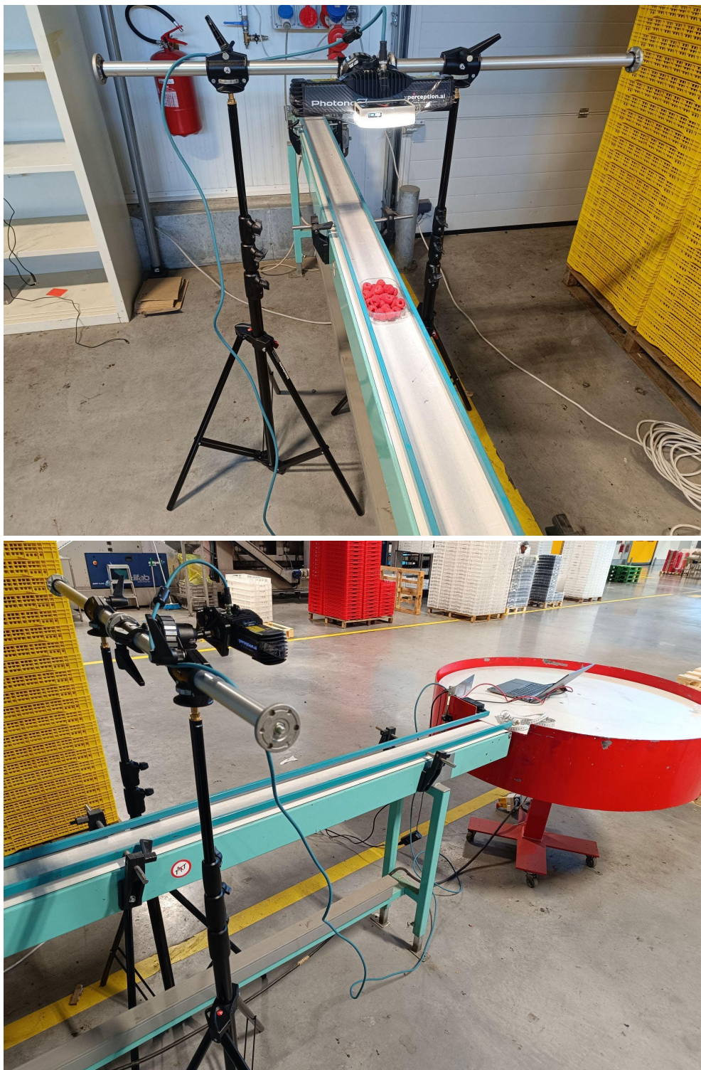
Figure 2. Grading system acquisition setup for raspberry grading.
