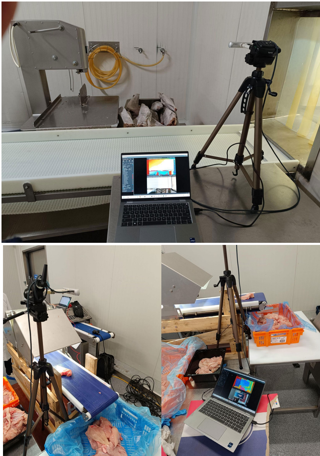
Figure 1. Grading system acquisition setup for fish, chicken and orange grading.
